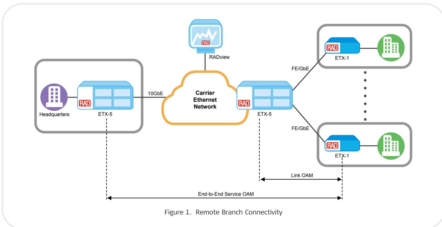
Figure 1. Remote Branch Connectivity
