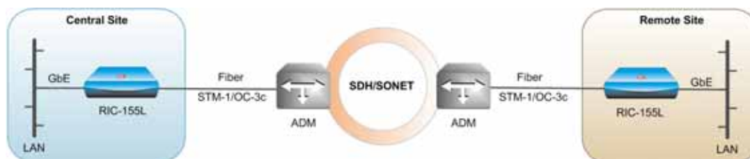
Figure 2. Point-to-Point Ethernet Private Line over SDH/SONET
