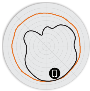
Figure 2. C110 2.4GHz Azimuth Antenna Patterns
